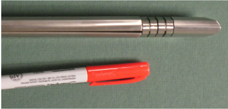
Figure 6.9: Photograph of buncher electrodes, with pen for scale.
